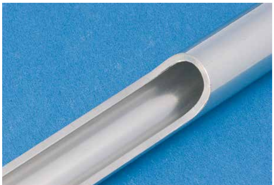
TPS standard SBS Level 2: bright annealed surface outside inside roll polished and bright annealed roughness outside Ra max. 0,8 µm | roughness inside Ra max. 0,8 µm
