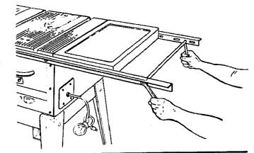
IMPORTANT: Apply a coat of paste wax to the top surface and front edge of the front guide bar. This will allow the fence to slide more easily.
