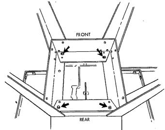
If you mount the saw on any other bench, make sure that there is an opening in the top of the bench the same size as the opening in the bottom of the saw so that the sawdust can drop through. Recommended working height is 33 to 37 in. from the top of the saw table to the floor.
