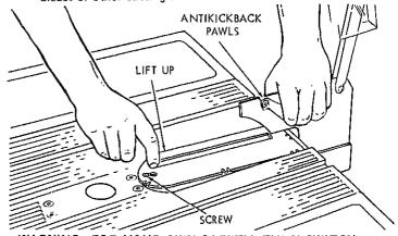
WARNING: FOR YOUR OWN SAFETY, TURN SWITCH "OFF" AND REMOVE PLUG FROM POWER SOURCE OUTLET BEFORE REMOVING INSERT.
