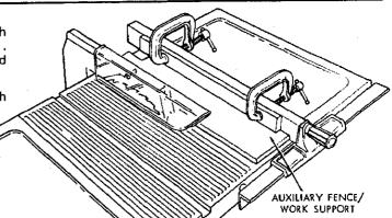
Feed the workpiece by hand along the AUXLIARY FENCE/WORK SUPPORT until the end is approx. 1 in. past the front edge of the table. Continue to feed using the PUSH BLOCK.
