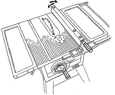
If the fence does not slide easily along the bars, the pressure of the spring can be REDUCED.
