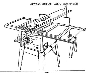
When "WIDTH OF RIP" is 6 in. and WIDER use your RIGHT hand to feed the workpiece until it is clear of the table.
