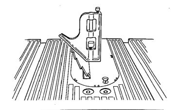
If blade is NOT  $45^{\rm o}$  to table . . . the  $45^{\rm o}$  STOP COLLAR and SCALE must be ADJUSTED
