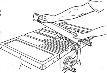
The rip fence must be PARALLEL with the sawblade and Miter Gauge grooves... Move fence until it is along side of groove. Do NOT LOCK IT. It should be parallel to groove. If it is not;
