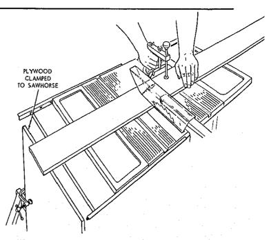
When using the RIGHT hand groove, hold the workpiece with your right hand and the lock knob with your left hand.
