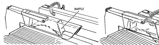
Narrow strips thicker than the Auxiliary Fence/Work Support may enter the guard and strike the baffle. CAREFULLY raise
