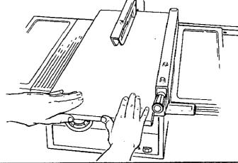
When "WIDTH OF RIP" is 2 in. to 6 in. wide USE THE PUSH STICK to feed the work.
