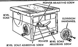
If blade is NOT SQUARE to table . . . the  $90^{\rm o}$  LIMIT STOP must be ADJUSTED.
