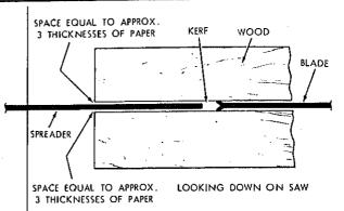
8. Make two folds in a small piece (6 x 6 in.) of ordinary NEWSPAPER making three thicknesses. The folded paper will be used as a "spacing gauge".
