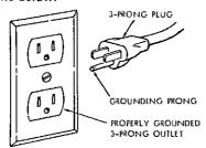
Plug power cord into 110-120V properly grounded type outlet protected by a 15-amp, time delay or Circuit-Saver fuse or circuit breaker.
