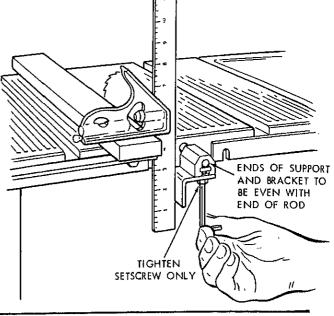
IMPORTANT: The SPREADER must always be PARALLEL to the sawblade and in the MIDDLE of the cut (KERF) made by the sawblade.
