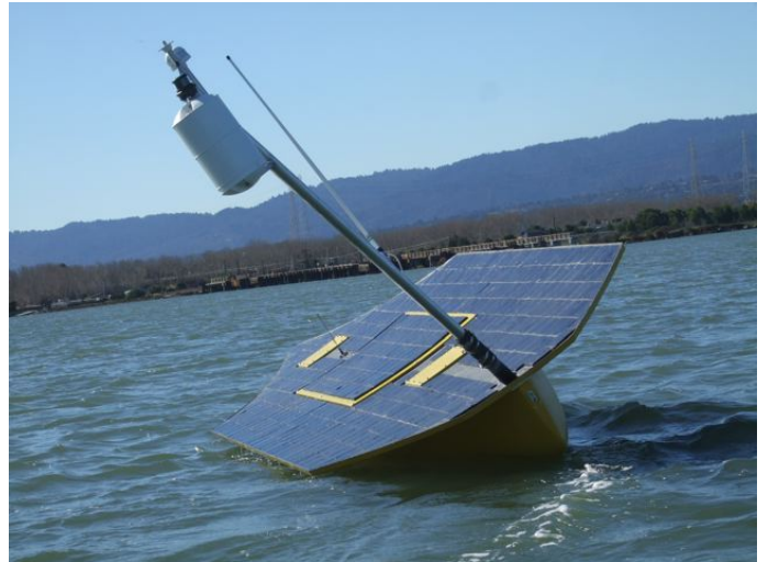
Fig. 1. An open-ocean test of autonomous control of the SeaSlug where the vehicle is controlling both heading and roll angle. Prominently displayed are its solar panels and radar reflector.
