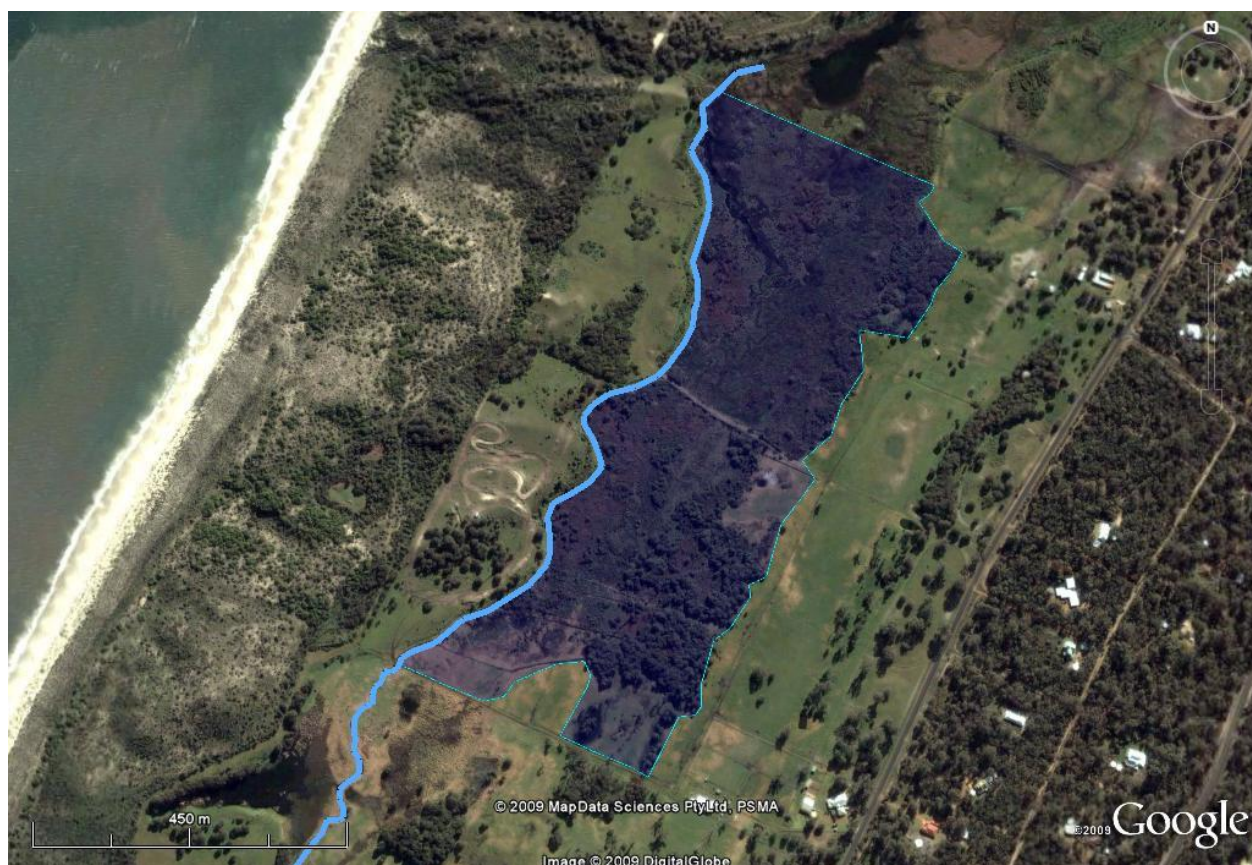
Figure 7. Hydrologic map of Muddy Lake: blue shaded region shows extent of seasonal waterlogging or inundation; the main drain, shown in light blue, runs along the eastern edge of the wetland and flows south (Google Earth 5.0)
