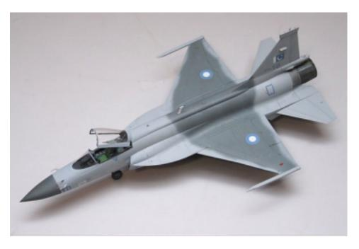
other rough bits that will take some attention to clean up. Panel lines and some fastener details might be a little heavy for some, but are consistent and cross few assembly joints that might risk being obscured by sanding or putty. The kit has separate control surfaces. Rudder, flaps, ailerons, and leading edge flaps, fit well, but the speed brakes, not separate, are not really differentiated from the basic panel lines.
