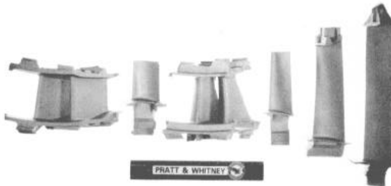
Figure 11 - PWA 1484 has been cast in a wide variety of airfoil configurations.
