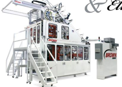
*Elite Series* Servo Driven Horizontal Trim Presses are equipped with a multitude of innovative cutting edge features for achieving greater speeds, superior precision trimming, longer tool life, ease of maintenance and faster changeover times. The *Elite Series* is capable of high speeds in excess of 175 stokes per minute and fast changeover times of less than 30 minutes.
