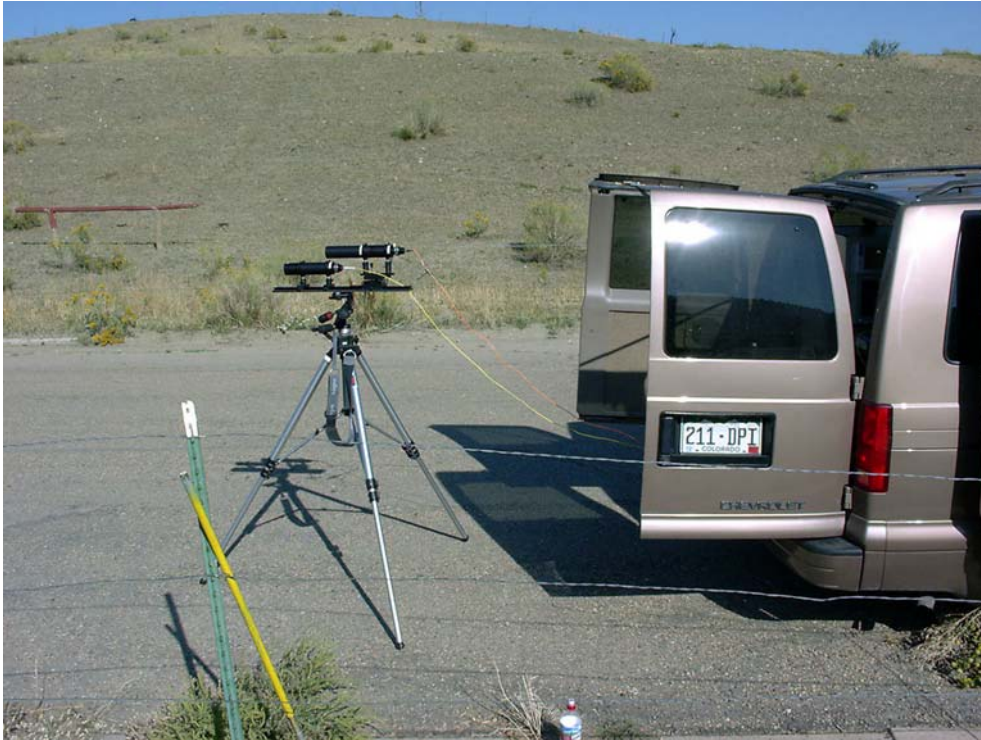
Figure 8. Photograph of the Laser Output and Signal Receiver 2-inch Optics Used in the Target Reflectance Tests
