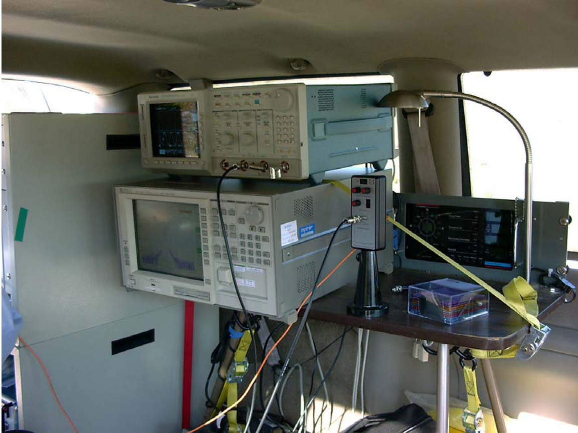
Figure 10. Test Equipment Located Inside Van for Target Reflectance Tests (Test Configuration Shown for Modulated Light Source Measurements)
