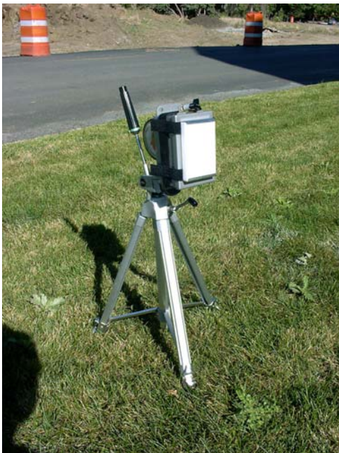
Figure 9. White Spectralon Target for Target Reflectance Tests
