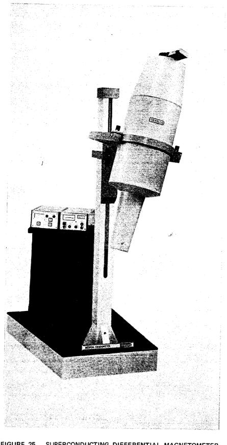
FIGURE 25 SUPERCONDUCTING DIFFERENTIAL MAGNETOMETER
