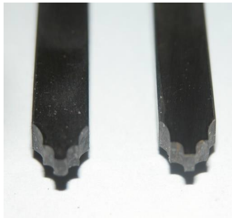
Another look from the front. Note the front relief corners. the Rounded on the left cutter and square on the right cutter. For some of us, our hands are not perfect machines. So, when stoning their full length, it might be challenging to maintain constant, square surface contact. Thus, at a minimum, keep your focus on the first 1/3 of the corner to ensure its surface maintains contact with the stone as this is the key area of the form cutter.
