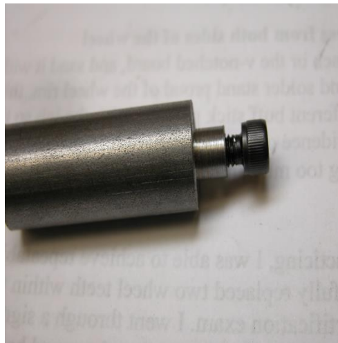
Quality check: finished arbor with its Allen screw
