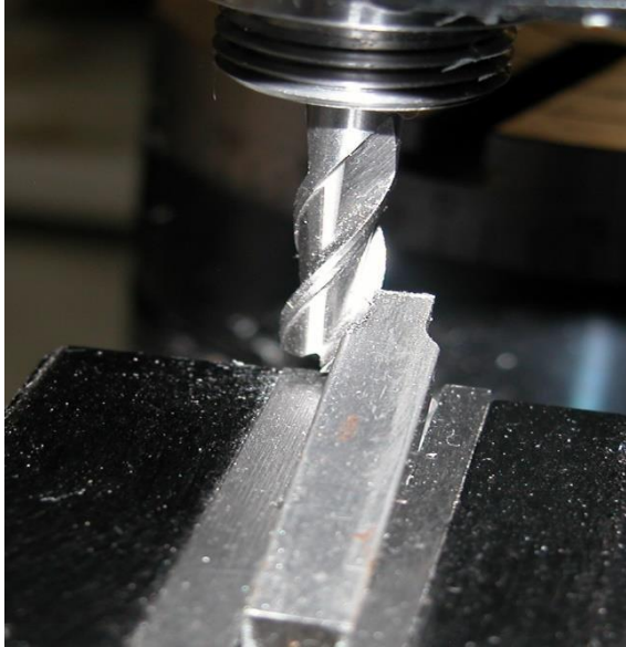
End mill is then traversed into the side of the cutter Distance C.
