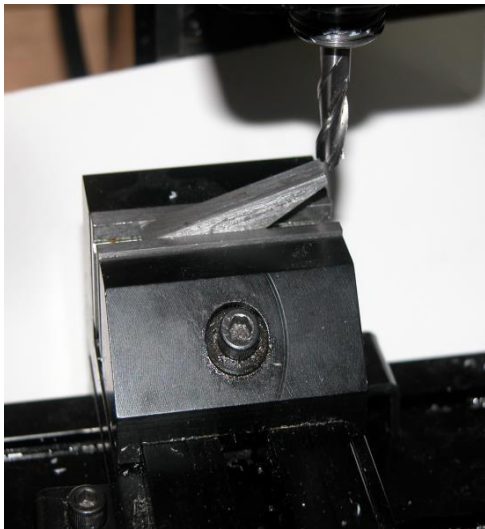
End mill is positioned to machine front relief square. Once front relief is machined square, establish zero position for the front relief as described above. Milling machine is then turned off.
