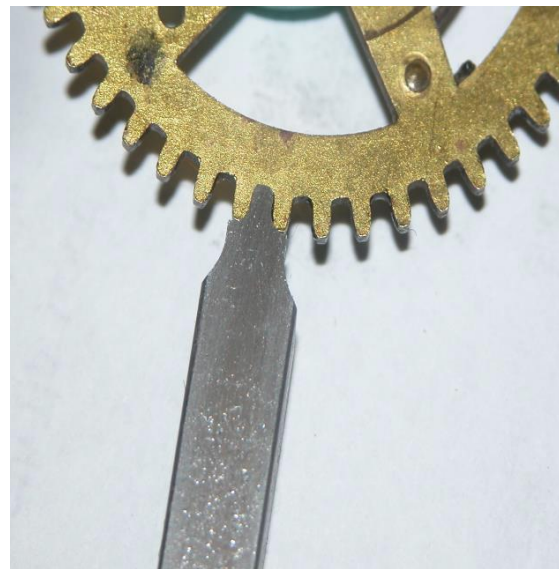
Notice that the tooth spaces have round bottoms. The two sharp corners on the cutter's front relief's needed to be stoned and rounded to complete the fit. Now we are done ☺.
