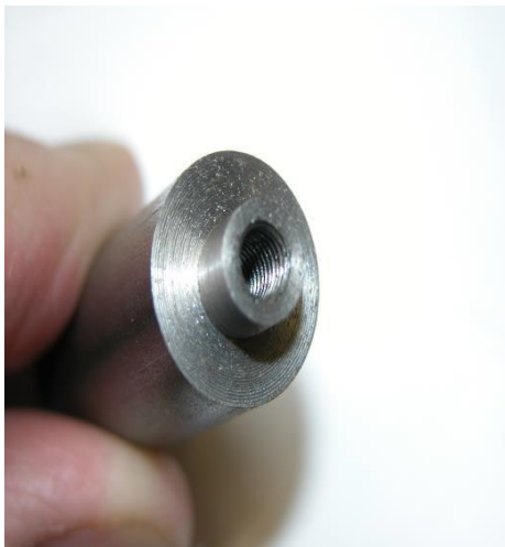
Arbor with internal threading
