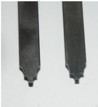
On the left is a cutter with a rounded tip and on right is a square cutter tip. A top down look.
