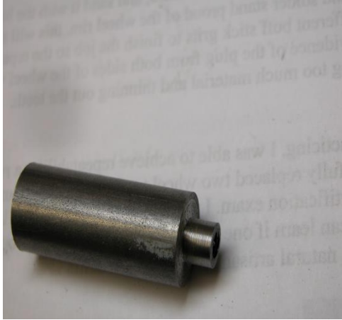
Step machined on arbor
