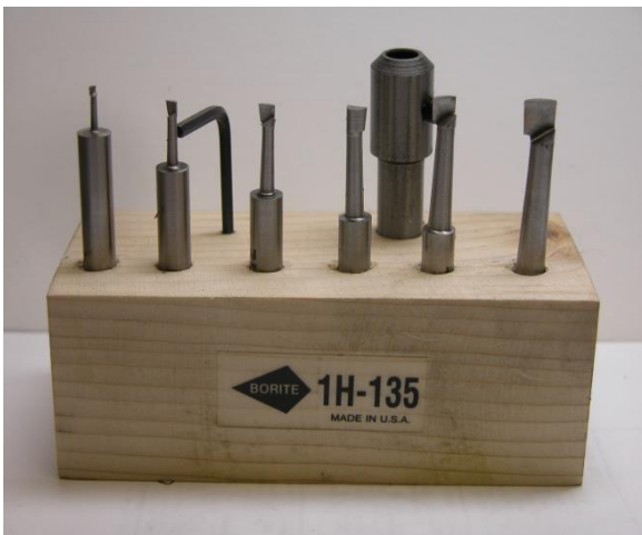
Borite HSS micro boring bar set from 1/16" – 1/4". Solid carbide is deemed a better boring bar tool as it is more rigid than HSS but it exceeded my pocketbook ☺.
