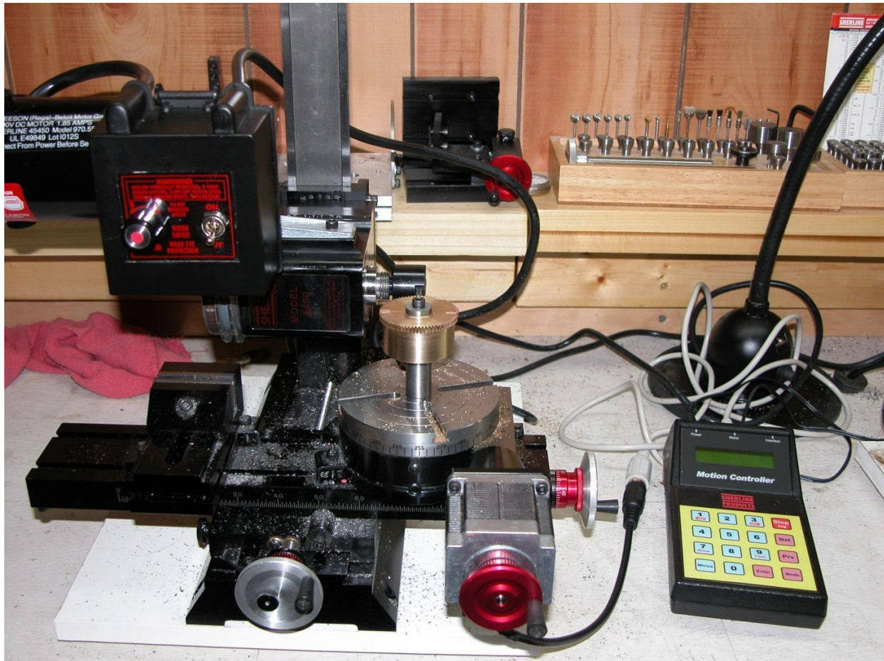
Machinist Vise, RT & CNC programmer setup. Note this setup is for a mainspring barrel. It is the same setup for a wheel blank.
