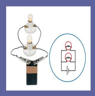
When light bulbs are connected in parallel, charges have more than one path to follow. The circuit can be complete even if one light bulb burns out.
