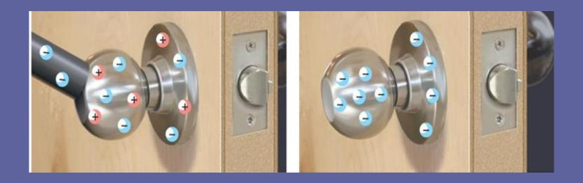
When a negative rod touches a neutral doorknob, electrons move from the rod to the doorknob.
