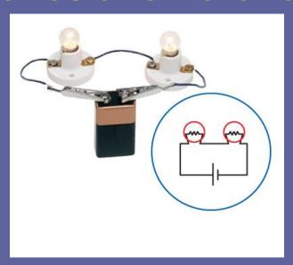
When light bulbs are connected in series, charges must pass through both light bulbs to complete the circuit.
