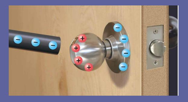
A negatively charged rod brought near a metal doorknob induces a positive charge on the side of the doorknob closest to the rod and a negative charge on the side farthest from the rod.
