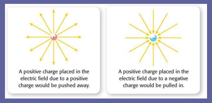
The electric field lines around a positive charge point outward.
