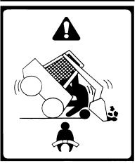
6. WARNING: KEEP CLEAR OF MOVING PARTS. KEEP BYSTANDERS CLEAR OF THE LOADER AT ALL TIMES UNLESS THE BOOM IS DOWN ON THE GROUND OR THE BOOM IS RESTING ON THE BOOM LOCK PINS AND ENGINE IS OFF. NEVER EXTEND ANY PART OF THE BODY OUTSIDE OF THE OPERATOR'S AREA.
