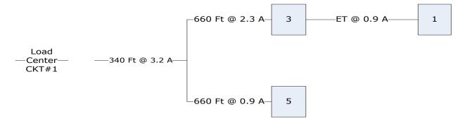
Circuit voltage is 240 volts.
