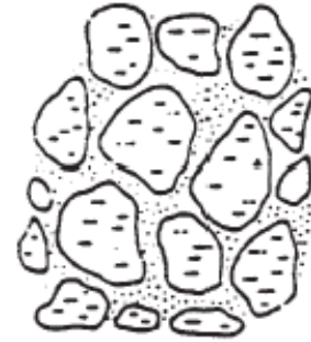
Aggregate with High Amount of Fines (>30 percent)
