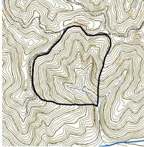
Figure 14b. Rotated topographic map and outline of convergent headwall displayed in the stereo pair of Figure 14a (Hunger Mountain and Snider Peak USGS 7.5' quadrangles).
