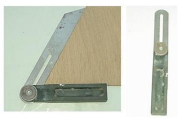
The knob tightens to hold the angle measured (left) The tool folds up to hang on a hook (right).
