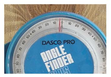
Above - Measuring the 3 degree down angle of the A/C box at the rear of the trailer.
