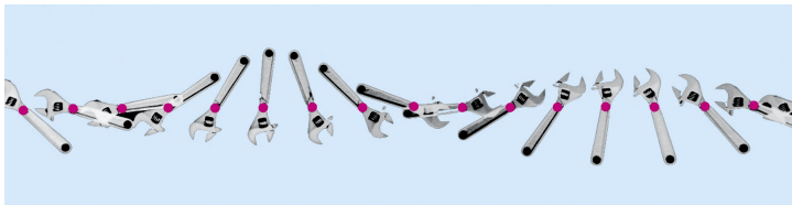
FIGURE (a) The motion of this wrench gliding on ice seems haphazard until we notice that the wrench is simply turning about its center of mass as the center glides in a straight line. (b) The planets, asteroids, and comets of our solar system revolve about their collective center of mass. (It lies inside the sun.)
