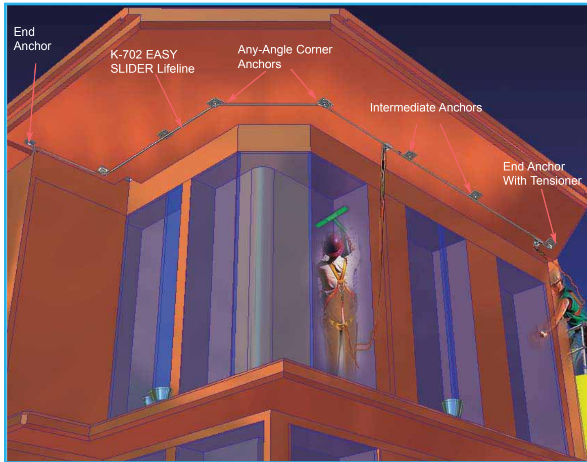
K-702 EASY SLIDER Horizontal Lifeline Provides Fall Protection For Window Cleaning
