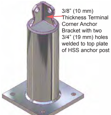
K-FARA-2-700-706 Start And End Corner Anchor
