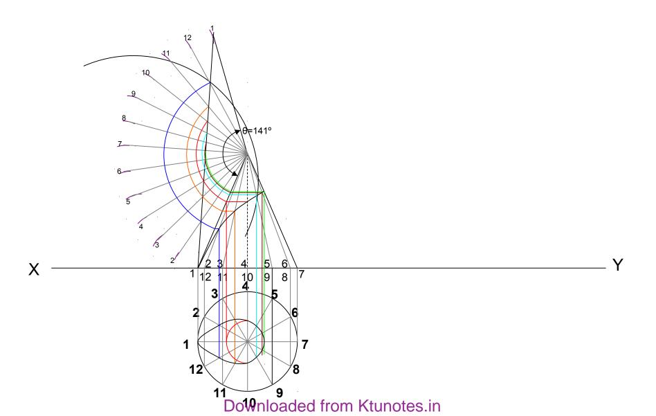
Q 15.26: A right circular cone base 30 mm side and height 50 mm rests on its base on H.P. It is cut by a section plane perpendicular to the V.P., inclined at 45° to the H.P. and bisecting the axis. Draw the projections of the truncated cone and develop its lateral surface.
