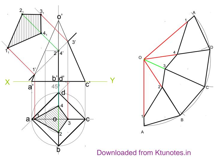
Q 15.26: draw the projections of a cone resting on the ground on its base and show on them, the shortest path by which a point P, starting from a point on the circumference of the base and moving around the cone will return to the same point. Base ofn cone 65 mm diameter ; axis 75 mm long.
