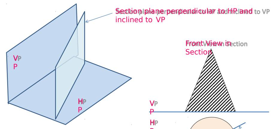
Sectionaplane endicular perpendicularto VP to HP and inclined to VP
