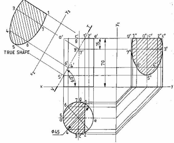
Note: <u>true shape of a section</u>: when the section plane is inclined, the section has to be projected on an auxiliary plane, parallel to the cutting plane, to obtain its true shape. Downloaded from Ktunotes.in
