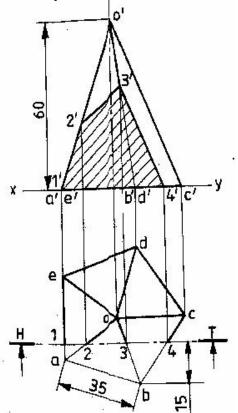
**NOTE:** True shape of a section: the projection of the section on a plane parallel to the section plane, will appear in its true shape of the section. Thus, when the section plane is parallel to H.P, the true shape of the section will be seen in the sectional top view. When it is parallel to V.P, the true shape of the section will appear in the sectional fron Dviewloaded from Ktunotes.in
