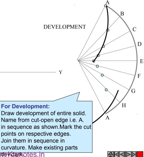
Q 14.11: A square pyramid, base 40 mm side and axis 65 mm long, has its base on the HP with two edges of the base perpendicular to the VP. It is cut by a section plane, perpendicular to the VP, inclined at 45° to the HP and bisecting the axis. Draw its sectional top view and true shape of the section. Also draw its development.
