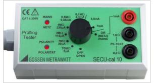
All limit values for the required tests per DIN VDE, as well as protective conductor resistance, insulation resistance, equivalent leakage current, differential and/or contact as well as housing leakage current must be tested.
