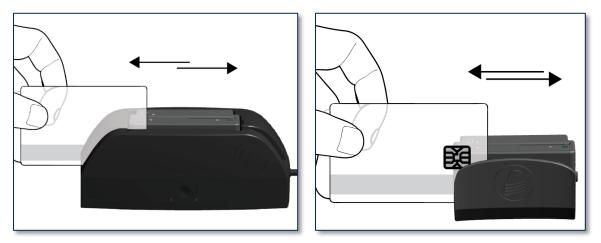
Figure 4-1 - Swiping a Card Through eDynamo
