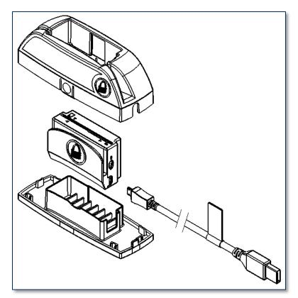
Figure 3-4 - Optional Docking Station Assembly
