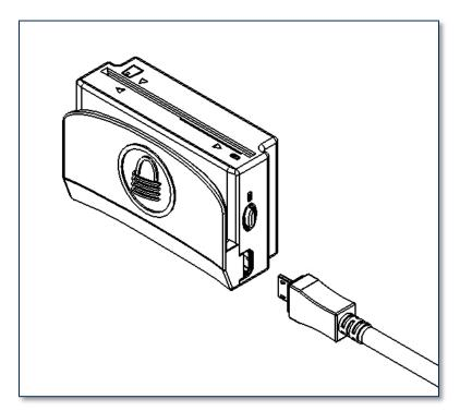
Figure 3-1 - Connecting eDynamo to a Computer
