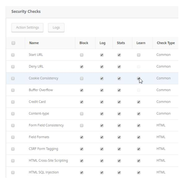
The screenshot above shows the required settings for Common and HTML checks. Some of the checks are not enabled for blocking, as they check for behaviours that may overlap with the normal behaviour of E-Business Suite, blocking which would interfere with the normal operation of these applications. However, any such instances are logged for later auditing.
