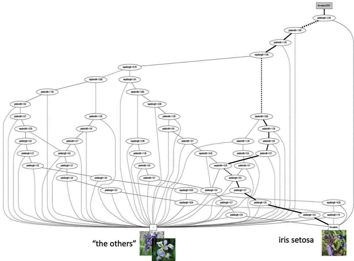
FIGURE 3. Class characterization. This Class Characterization Model has only 53 nodes, a size that can be considered comprehensible by humans. Its maximal path length is 18. The path for our sample is 14, and the corresponding reduction leads to an outcome explanation with only 4 predicates. Note that with four classification parameters the outcome explanation can never have more than 4 predicates.
