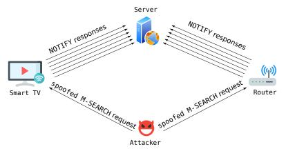
Figure 2. Example of SSDP amplification/reflection DDoS attack toward a server.
