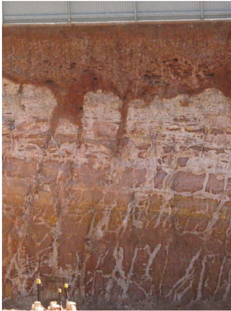
Figure 4.13 Weathering profile upon a red calcareous mudrock. Northern Territories, Australia.
