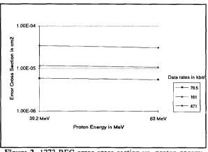
Figure 2 1773 REC error cross-section vs. proton energy for each data rate
