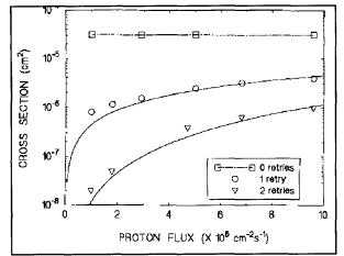
Figure 8 1773 REC error cross-section vs. flux for 0,1,2 retries
