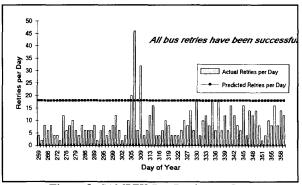
Figure 9 SAMPEX Bus Retries per Day
