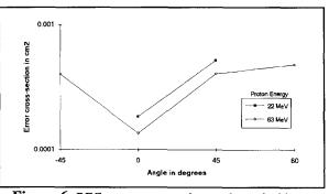
Figure 6 REC error cross-section vs. beam incidence angle
