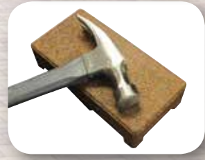
AZEK PAVER AFTER BEING HIT WITH HAMMER
