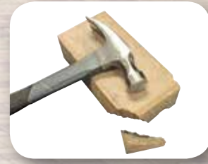
CONCRETE PAVER AFTER BEING HIT WITH HAMMER
