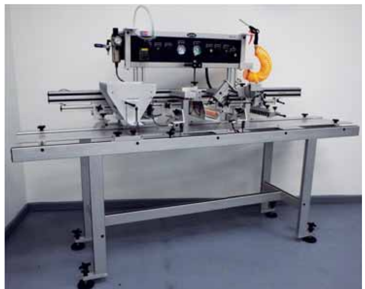
Figure 13-16. This automatic needle seeder can be adjusted to sow different sized seeds.
