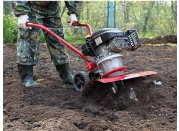
Figure 13-9. A tiller can be used to till and crumble the soil in the same manner as a field tractor.
