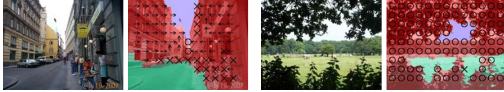
Figure 3.1: Surface layout. In these images and elsewhere, main class labels are indicated by colors (green=support, red=vertical, blue=sky) and subclass labels are indicated by markings (left/up/right arrows for planar left/center/right, ‘O’ for porous, ‘X’ for solid).
