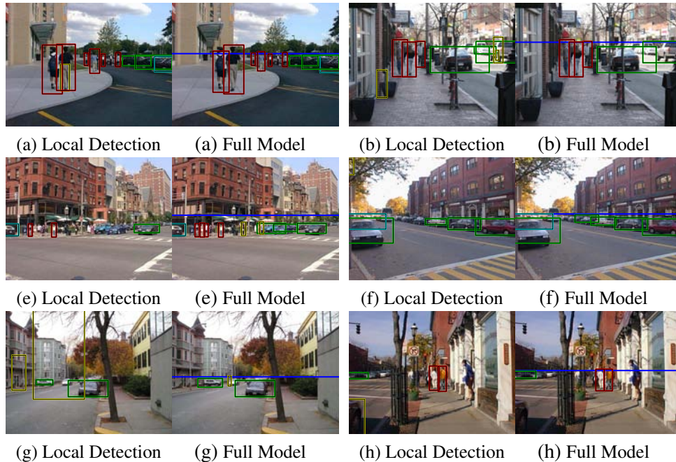
Figure 5.11: We show local object detections (left) of Dalal-Triggs (green=true car, cyan=false car, red=true ped, yellow=false ped) and the final detections (right) and horizon estimates (blue line) after considering surface geometry and camera viewpoint (initially estimated using our scene matching method). Our method provides large improvement (+7%/11% for peds/cars at 1 FP/image) over a very good local detector. Many of the remaining recorded “false positives” are due to objects that are heavily occluded (a,e) or very difficult to see (e) (i.e., missed by the ground truth labeler). In (h), a missed person on the right exemplifies the need for more robust assumptions (e.g., a person usually rests on the ground plane) or explanation-based reasoning (e.g., the person only looks so tall because he is standing on a step).
