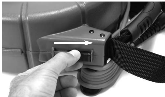
Figure 4 – Unlatching the microReel Case
