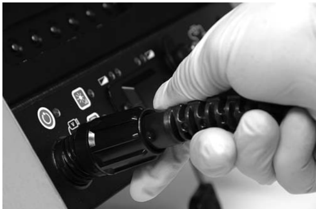
Figure 13 – Connecting To A SeeSnake CCU
