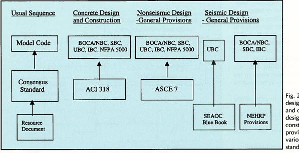
Fig. 2. Seismic design provisions and concrete design and construction provisions in various codes and standards.
