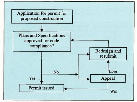
Fig. 1a. Issuance of construction permit.
