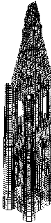
Figure 9 Finite element model of the tower
