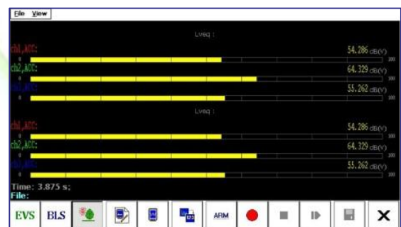
3-axis Environmental Vibration mode by JIS C 1510
