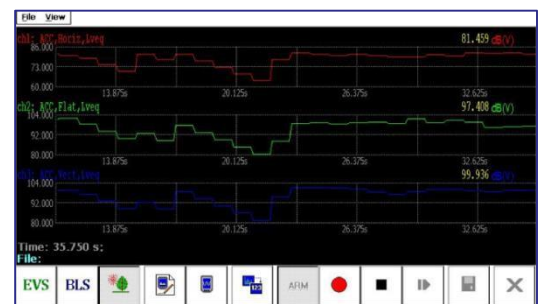
Environmental Vibration mode by JIS C 1510
