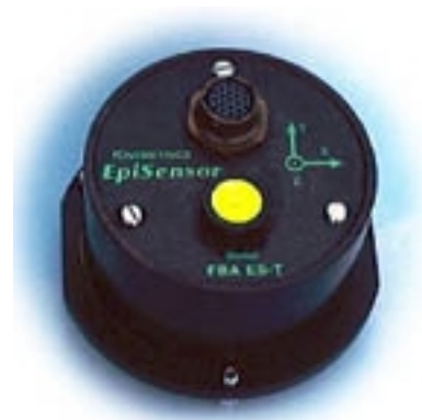
Figure A-2. Triaxial Episensor (13.3 cm diameter, 6.2 cm height)
