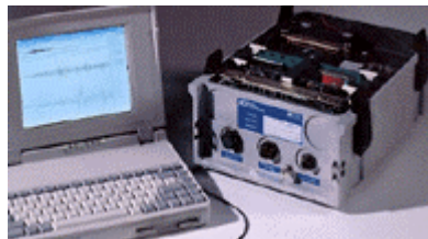
Figure A-4. Modern digital K-2 recording system can download data to a laptop or transfer by modem or other communications media.
