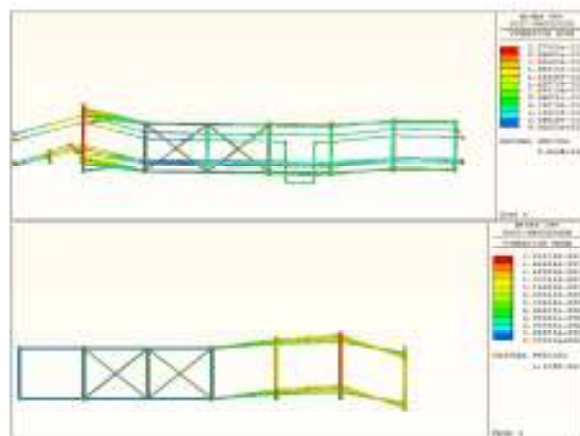
Figure 4.3. Main vibration mode with and w/o pipes.
