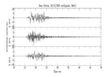
Fig. 2. The accelerographs of the Bam earthquake
