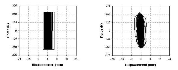
Figure 10. Hystereses for peak table acceleration of 0.35g in X-direction of the piping system
