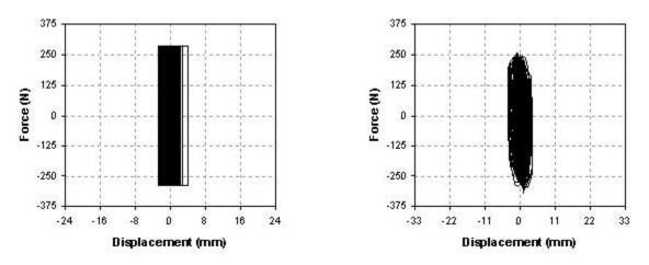
Figure 14. Hystereses for peak table acceleration 0.29g in Z-direction of the piping system
