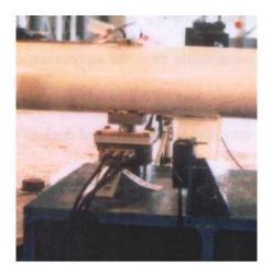
Figure 2. Photograph of the friction damper
