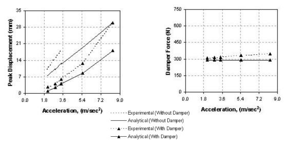
Figure 7. Seismic response in Z-direction of piping system with friction damper
