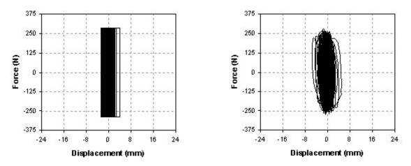
Figure 9. Hystereses for peak table acceleration of 0.27g in X-direction of the piping system
