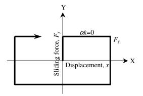
Figure 5. Hysteresis for friction damper represented by Wen's model
