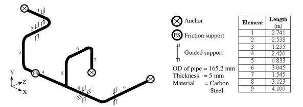
Figure 4. Schematic diagram of the piping system with friction damper
