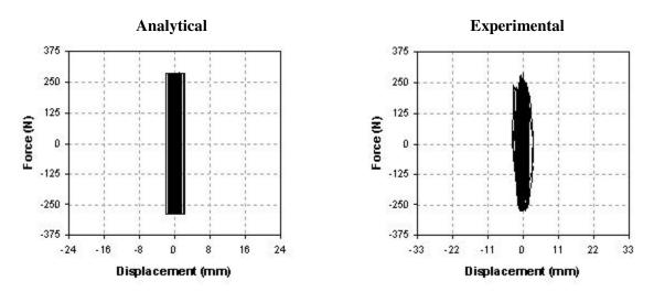
Figure 8. Hystereses for peak table acceleration of 0.2g in X-direction of the piping system
