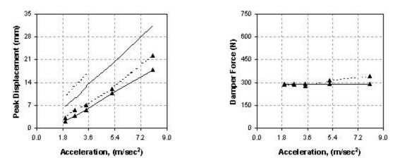
Figure 6. Seismic response in X-direction of piping system with friction damper
