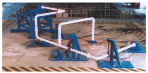
Figure 3. Test setup of the piping system with friction damper
