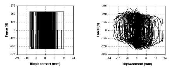
Figure 12. Hystereses for peak table acceleration of 0.82g in X-direction of the piping system
