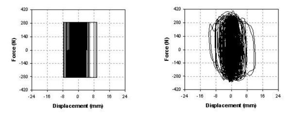
Figure 11. Hystereses for peak table acceleration of 0.53g in X-direction of the piping system
