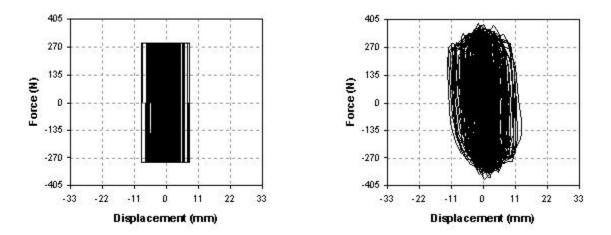
Figure 16. Hystereses for peak table acceleration of 0.56g in Z-direction of the piping system
