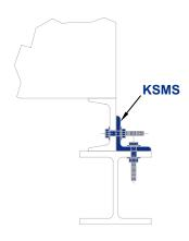
Model KSMS (detail left) seismic and wind restraint brackets are used to solid-mount equipment to the building structure. It can be bolted or welded to the equipment, and is attached to the structure by anchoring to concrete or bolting to steel.
