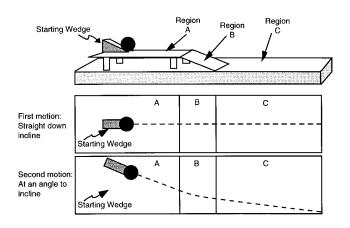
Fig. 3. Apparatus used in the tutorial entitled *Changes in Energy and Momentum* that helps students learn to apply the work-energy and impulsemomentum theorems. The ball is released from the same height on the starting wedge in the two cases.
