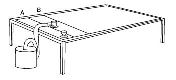
Fig. 2. Apparatus used in individual demonstration interviews on workenergy and impulse-momentum tasks. Students are asked to compare the final momenta and kinetic energies of two dry-ice pucks (one brass and one plastic) that move on a glass table. A constant force is applied by a steady stream of air in a direction perpendicular to the two parallel lines. Each puck starts from rest at line A and moves, without rotating and essentially without friction, to line B.
