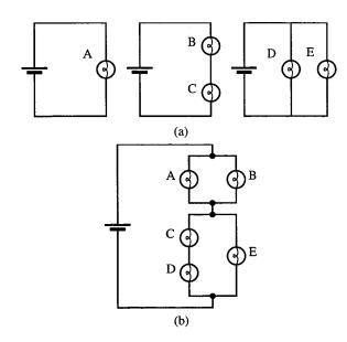
Fig. 1. Circuits used on questions given (a) after standard instruction on electric circuits and (b) after students had studied the material through guided inquiry. Students are asked to rank the bulbs from brightest to dimmest and to explain their reasoning. In both cases, they are told to treat the bulbs as identical and the batteries as identical and ideal.
