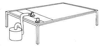
Fig. 1. Apparatus for momentum and energy comparison tasks. Two dryice pucks move without friction on a level glass table. Equal force is applied to the two pucks by a reversed vacuum cleaner as they move rectilinearly from line (a) to line (b).
