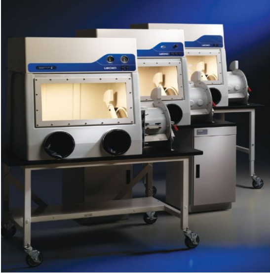
Figure 23 Photograph of Glove Boxes
