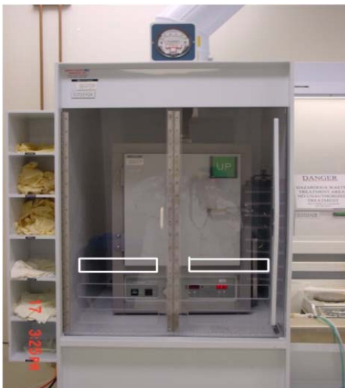
Figure 26 Photograph of Ventilated Equipment Enclosure
