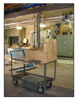
Figure 15: FLIR SC640 ThIR camera mounted on the cart for field demo.
