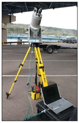
Figure 18: Typical Reigl LiDAR unit setup.
