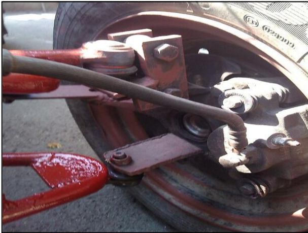
Fig.19 Front knuckle with attachment
