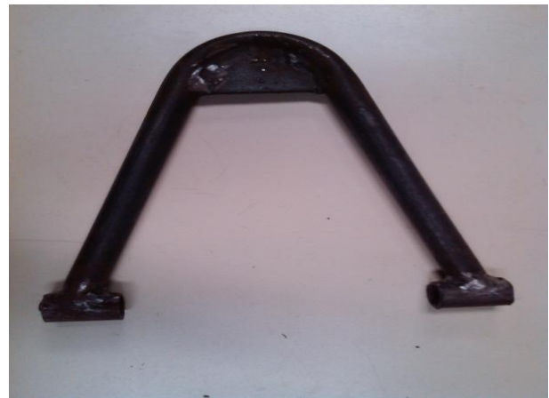
Fig.17. Fabricated front wishbone
