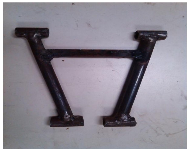
Fig.18. Fabricated rear wishbone
