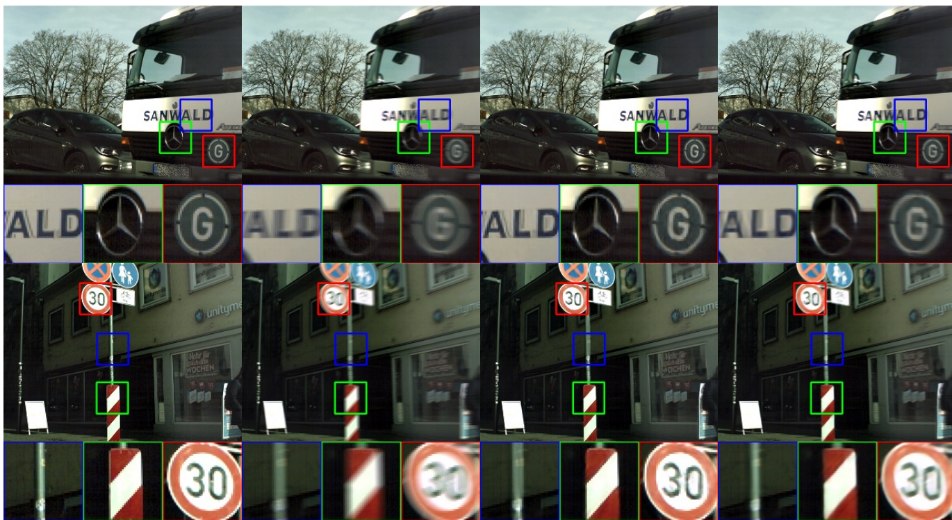
Fig. 4: Qualitative comparisons on synthetic dataset. First: Ground truth sharp image. Second: Input blurry image. Third: Deblurring results of the supervised method from Tao et al. [32]; The network is retrained on our dataset. Fourth: Deblurring results of the proposed self-supervised learning method.
