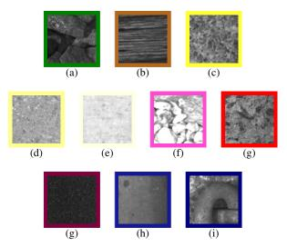
**Fig. 3.** Material categories. (a) ballast (b) wood (c) rough concrete (d) medium concrete (e) smooth concrete (f) crumbling concrete (g) lubricator (h) rail (i) fastener
