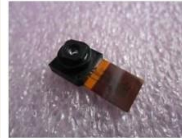
MT9V143M05STC DIGITAL IMAGE SENSOR 1/4 INCH VGA CMOS ACTIVE PIXEL Camera Chip
