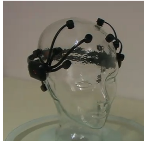
Fig. 4. Epoc neuroheadset from Emotive. The cap is connected wirelessly to the computer.
