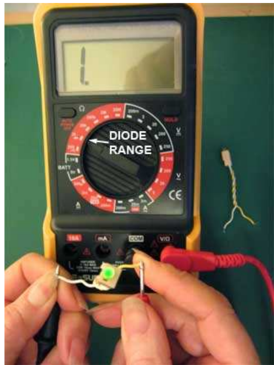
Figure 2.5.12. Testing a LED
