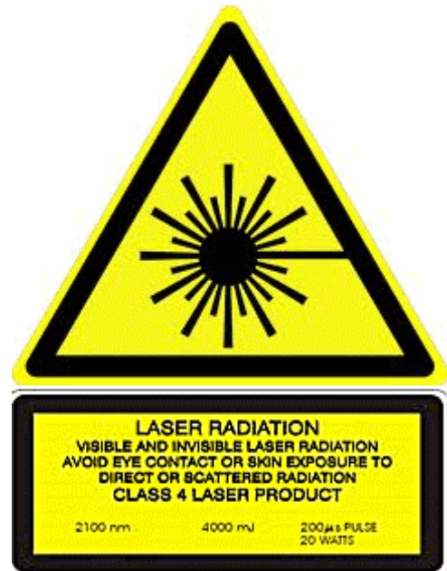
Fig. 2.6.9 Typical Laser Warning Stickers
