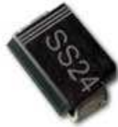
Figure 2.2.7. Surface Mount Schottky Rectifier in a DO-214 (5.3 x 3.6mm) Package
