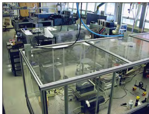
Figure 2. Laboratory for excimer laser energy and power meter calibrations, with measurement systems for 248 nm, 193 nm, and 157 nm. The excimer lasers are along the top right and the enclosures for nitrogen gas purging are in the foreground.
