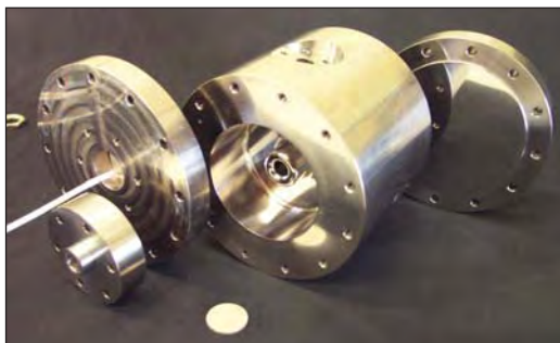
Figure 2. Second-generation acoustic viscometer made from Monel for use with corrosive gases.
