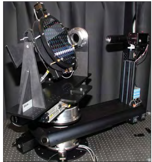
Figure 1. The new Goniometric Optical Scatter Instrument (GOSI) is a reference reflectometer for diffuse and specular scattering measurements having 300 mm sample capability.
