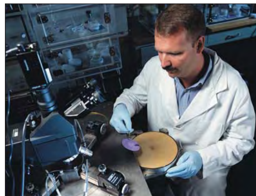
Figure 3. Curt Richter loads a molecular electronic sample for electrical characterization. Copyright Robert Rathe.
