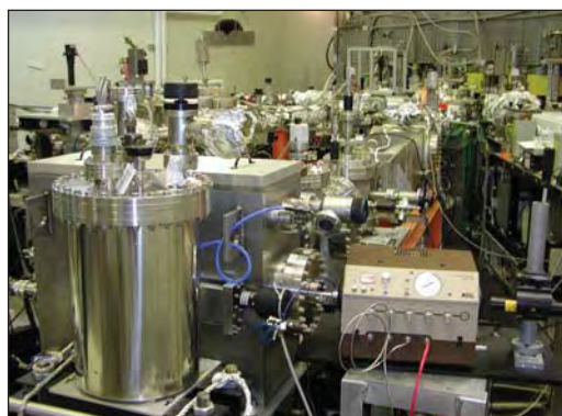
Figure 4. Measurement system for detector damage study by a 157 nm pulsed excimer laser.
