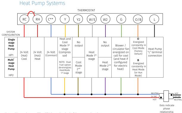
\*Internal jumper between RC and RH, located on back of thermostat above battery compartment.
