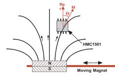
sors know the exact position and do not require indexing. Rare Earth magnets such as Neodymium or samarium cobalt types can be substituted with cost-effective Alnico or ceramic type magnets in typical applications such as linear displacement, angular displacement, motor control, and valve position.
