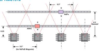
+/- 90 Degrees with a single HMC1512 Full 360 Degree Sensing with an Additional Hall Sensor
